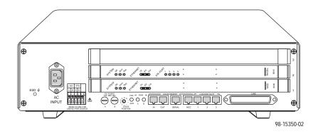
In a stacked configuration, the first or base chassis must contain an MCC card in Slot 1. In addition to the MCC card, the base chassis can house up to two DSL cards. Each additional chassis in the stack houses up to three DSL cards. For more information, see the *Hotwire 8600 Digital Subscriber Line Access Multiplexer (DSLAM) Installation Guide*.
